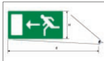
Figure 2 - Maximum viewing distance for Fire Safety signs
